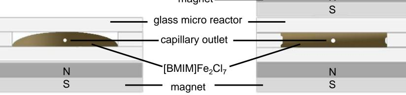
Observed shaping of the MILC inside the cavity under magnetic force. Single-sided mounted magnet gave a droplet-like shape with open spaces at the upper edges (left). A filled cavity appeared by applying two magnets on the opposite sides (right)
