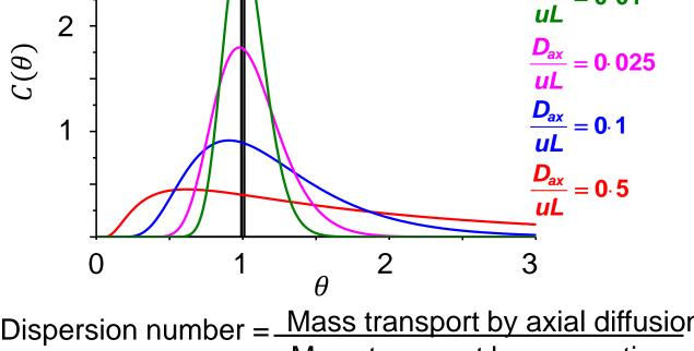
Dispersion becomes dominant for laminar flow in a tube reactors with a small diameter!
