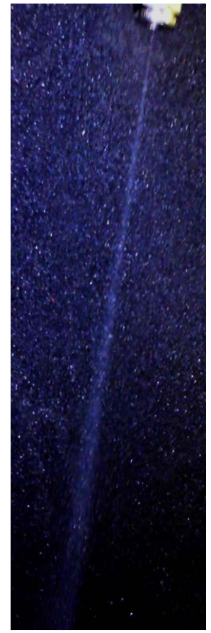
Free falling droplets, e.g. spray, encased by gas
